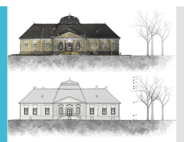
orthogonal point cloud and 2D facade view made based on it
